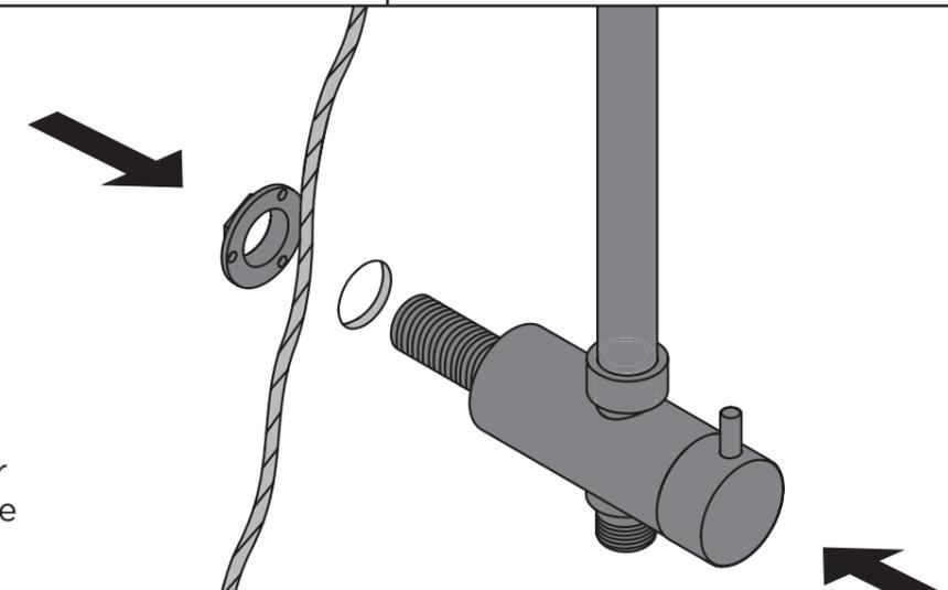
Secure the diverter to the wall using the backnut.
