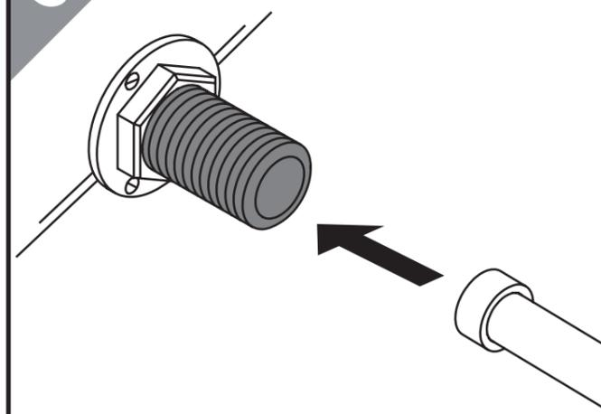
Connect water supply to the diverter inlet
