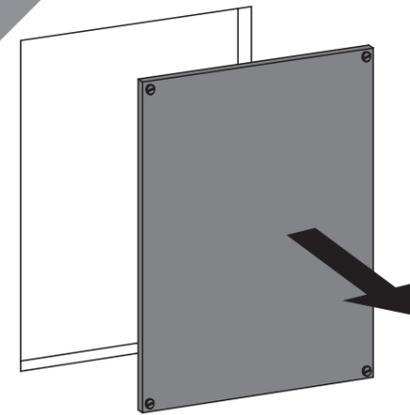
Prepare the pipework. Create the rear access point in the back of the wall cavity.
