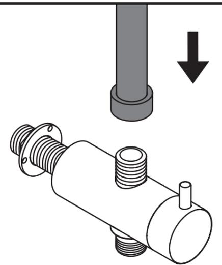
Ensure the olive is positioned correctly and attach the rigid riser to the diverter
