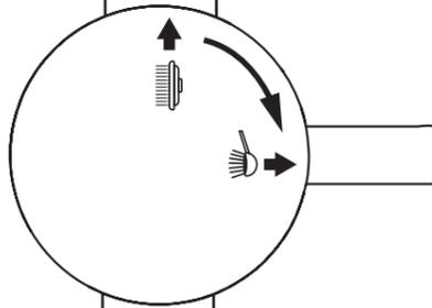
Turn the lever clockwise to direct water flow to the fixed head.
