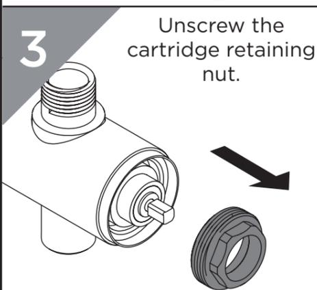
Unscrew the cartridge retaining nut.
