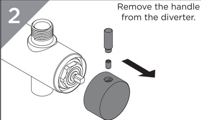
Remove the handle from the diverter.
