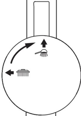
Point the lever upwards to direct water flow to the adjustable riser.
