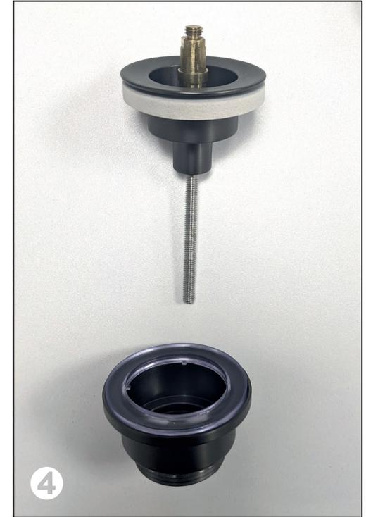
Unscrew the top cover to reveal the brass click-clack bracket. A stainless steel bracket will have also been included within the pack which can be switched with the brass bracket to ensure the waste stays open - usually used for basins without overflows.
