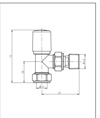
Dimensions (measurements in mm)
