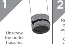
Remove the outlet and washer from housing. Clean and replace as necessary.
