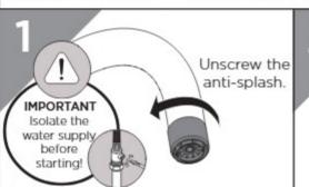
Remove the anti-splash and filter from housing. Clean and replace as necessary.
