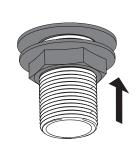
To secure the taps to the bath, use a box spanner to tighten the metal backnuts underneath ensuring the washer is correctly positioned in between the backnuts and the bath
