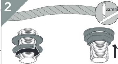
To secure the taps to the bath, use a box spanner to tighten the metal backnuts underneath ensuring the washer is correctly positioned in between the backnuts and the bath
