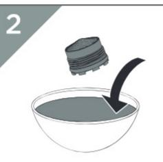
Check all loose parts for damage and then soak using a suitable solution to de-scale.
