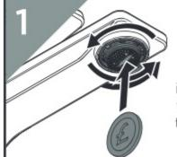
Insert a coin into the slot in the outlet and twist gently to remove.
