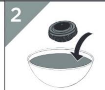
Check all loose parts for damage and then soak using a suitable solution to de-scale.
