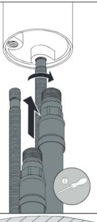
Thread the tap and tails through the plinth ensuring the rubber seal
