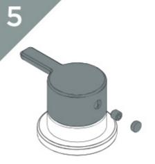
Replace the side body handles to secure in place.
