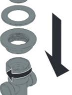
Feed the spout through the tap hole, ensuring the washer is in place.
