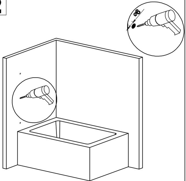
Dry fit required for best position to connect wall profile
