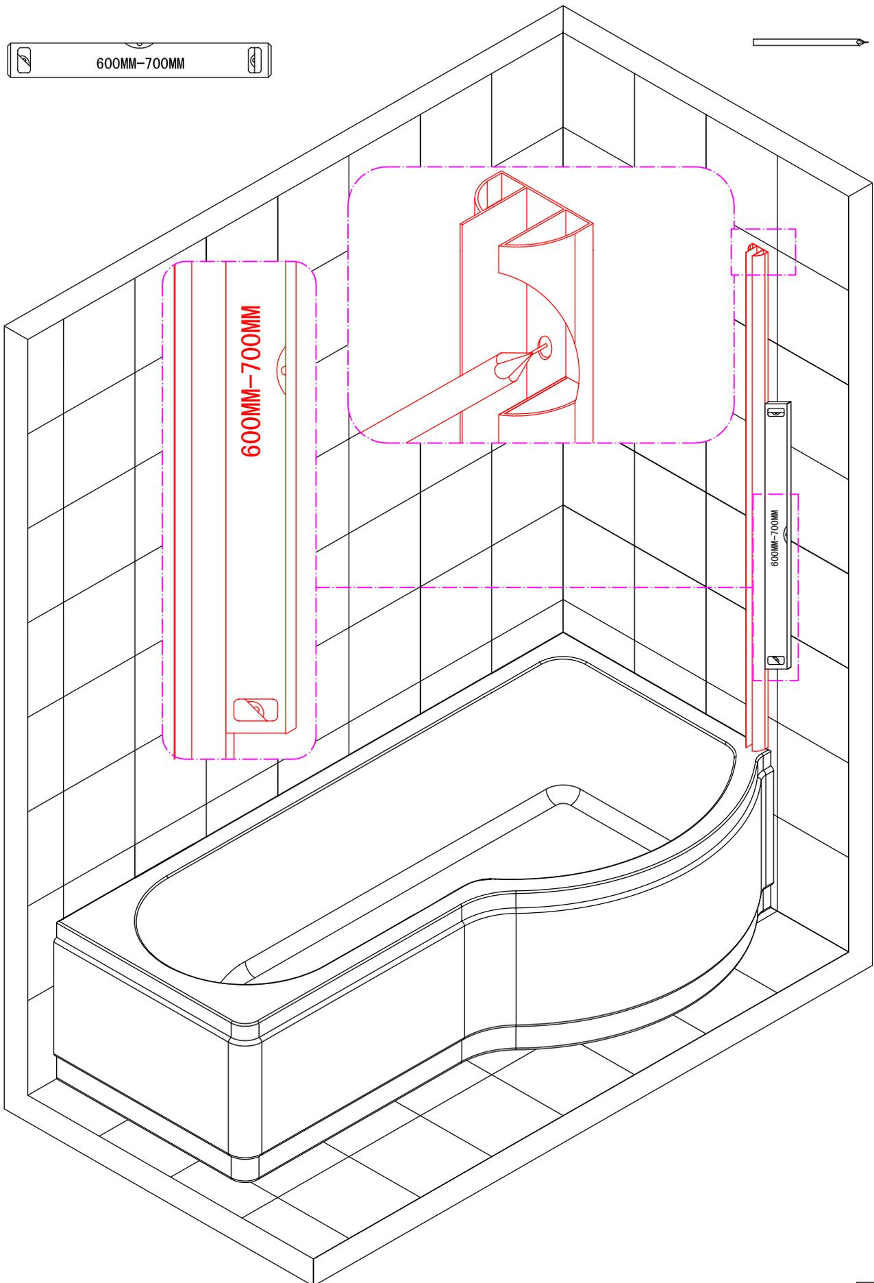
\*\*\*Dry fit required for best position to connect wall profile!\*\*\*
