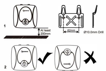
**IMPORTANT:** MS6 water heaters are designed for installation with the outlet / inlet pipes pointed upwards (to the ceiling). Under no circumstances should these units be fitted upside down, with the outlet / inlet pipes pointing towards the floor.(see diagram 2)
